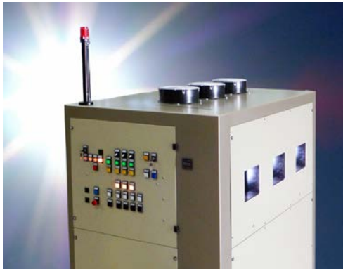
The compact sun simulator from Kinoton is used to reproduce the long-term effects of continuous exposure to sunlight.
